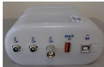
The module back provides two analog output connectors and one TTL output connection.
