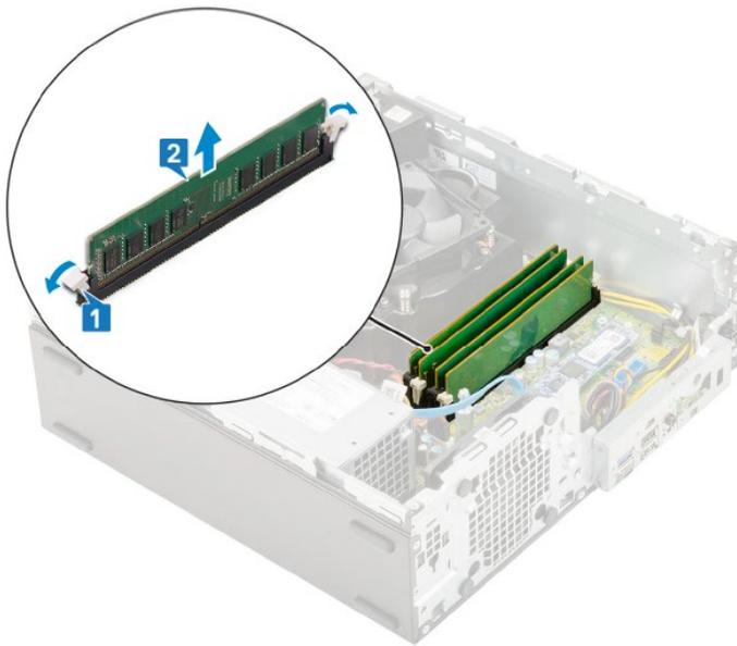
3. Install new RAM module by aligning the notch in the module with the tab on the RAM module connector.
