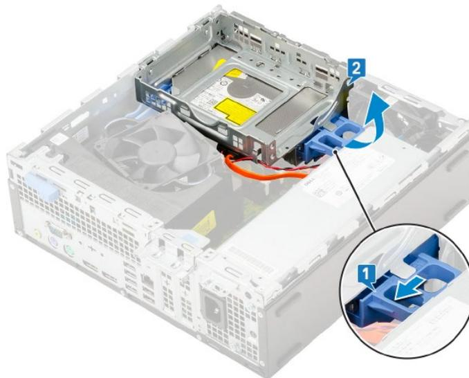
4. Once the cables are removed from the retainers, slide the chassis latch and lift the chassis assembly upwards, until it can be lifted off of the two hooks located on the side of the computer, as shown above right.
