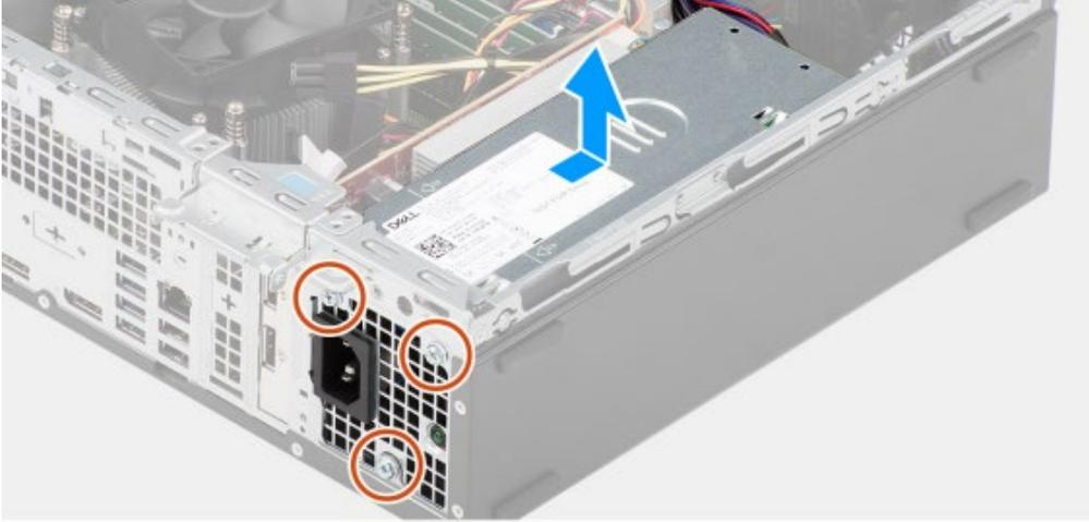
3. Slide the power-supply unit away from the back of the chassis.
