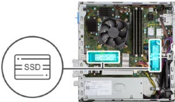
1. Remove the screw (M2x3) that secures the solid-state drive to the system board.
