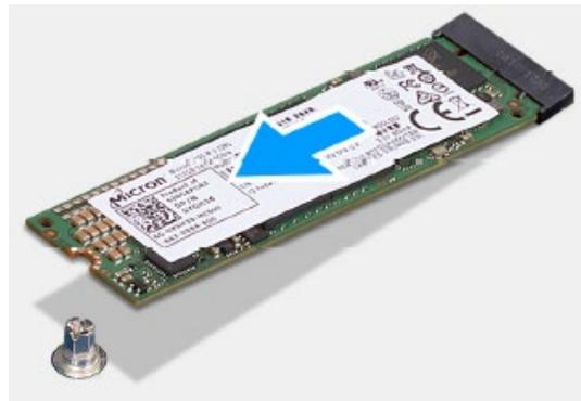
2. Slide at an angle to lift and remove the solid-state drive from its connector on the system board.
