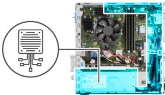
1. Disconnect the power cables from the system board and unroute them from the routing guides on the chassis.
