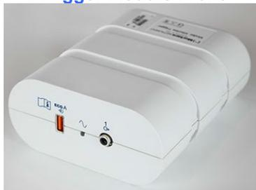
XScribe Front End is connected to the ECG A USB connector on the module front. One analog output connection is also on the front.
