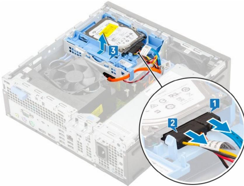
4. To remove the drive from the drive assembly, gently pull the two plastic retaining tabs outward to allow the drive to be slid out of the drive assembly.
