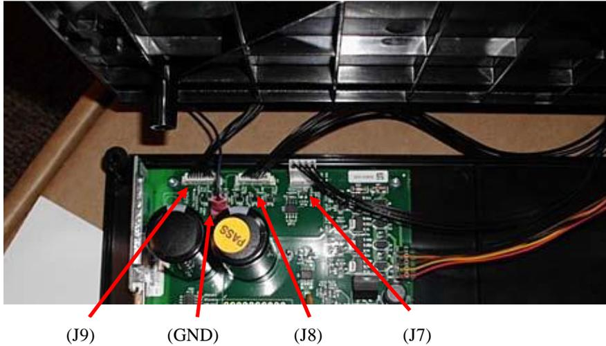
**CUE SENSOR CALIBRATION** – Required after replacement of motherboard, writer assembly, or cue sensor.
