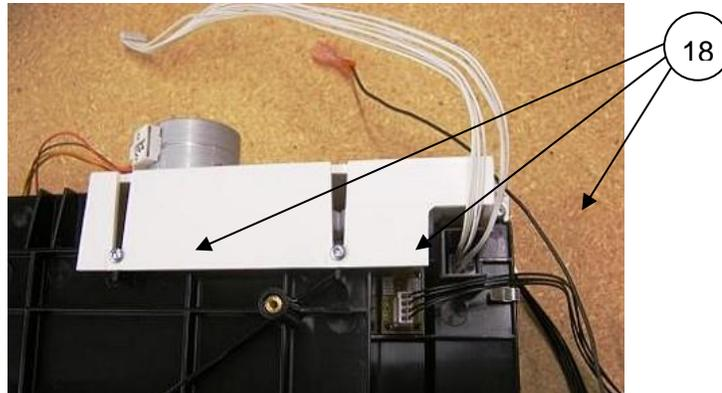
Remove the stepper motor from the *Gear Box* (Item 16) by removing 2 screws (17).
