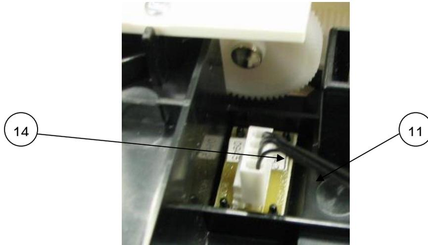
Two of the 4 plastic posts (A) that hold the Cue Sensor onto the Paper Tray (12) have a cyanoacrylate adhesive applied to hold it in place. Use a side cutter to flush cut the two posts with the adhesive to remove the Cue Sensor PCB (11) from the Paper Tray (use the two remaining posts to fasten the replacement item).
