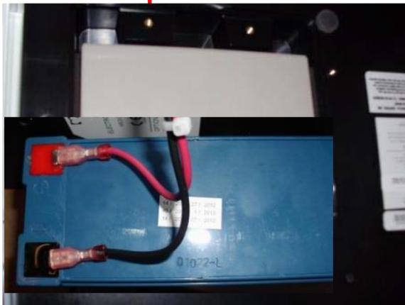
NOTE: Care must be taken when assembling the battery to connect the red wire to the red terminal and the black wire to the black terminal.
