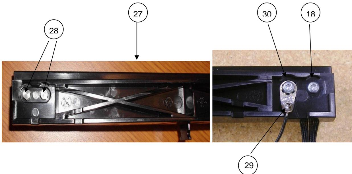
When reinstalling the printhead assembly, create a loop with the ground wire to allow it to move freely within the provided slot.
