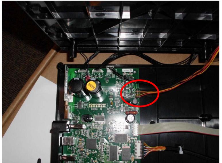
Continue to lift the Writer Assembly and remove J9, J7, J8 and the writer ground cable.
