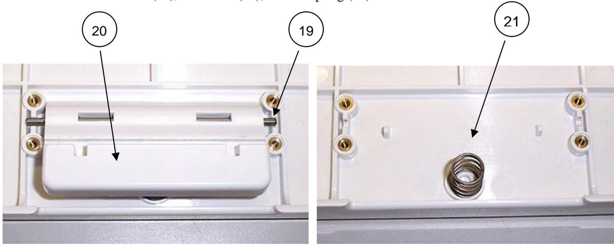
The picture below shows the writer assembly with the latch removed.
