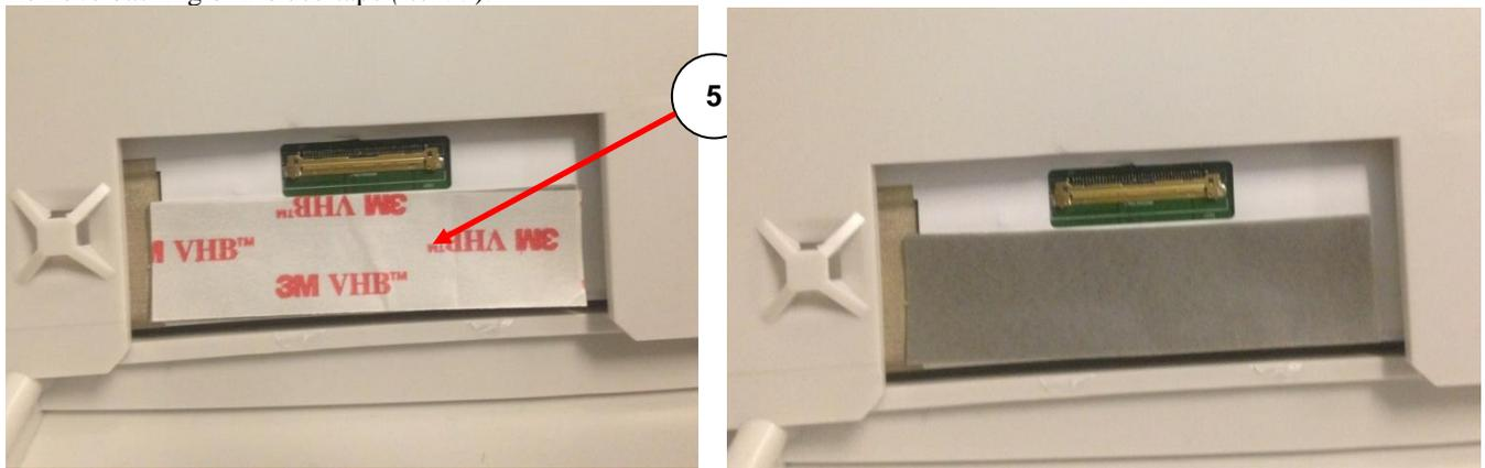
Install *Cable Assembly* (*Item 8*) into LCD connector at location CN1. Apply uniform pressure across Cable Assembly. Align Cable Assembly so the wires are positioned straight back from the connector as shown.
