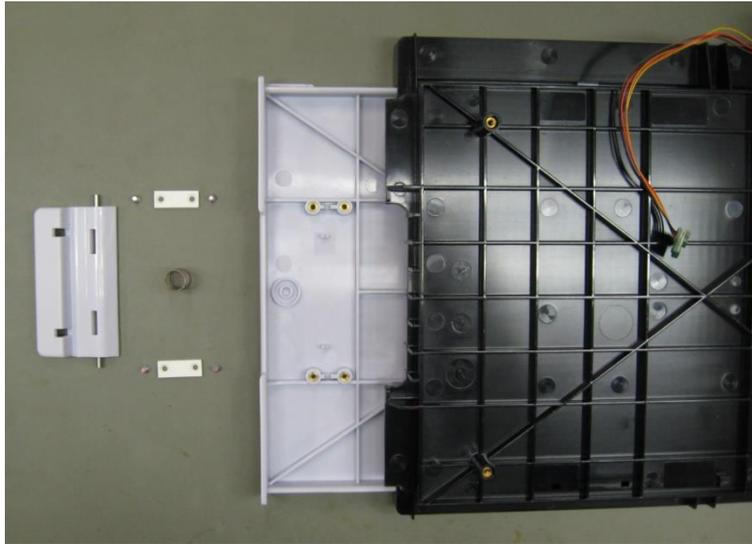
On the other end of the writer assembly, the printhead assembly must be removed from its installed position. This is done by removing the O-Ring that holds the assembly in place (underside of area circled) and unlatching the Spring Bar retaining clips as shown below.
