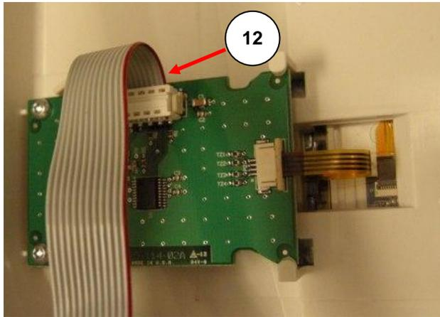
Unlock the flex cable connector by sliding the locking mechanism to the outward edge of the PCA (item # 14), then remove the flex cable from the connector.
