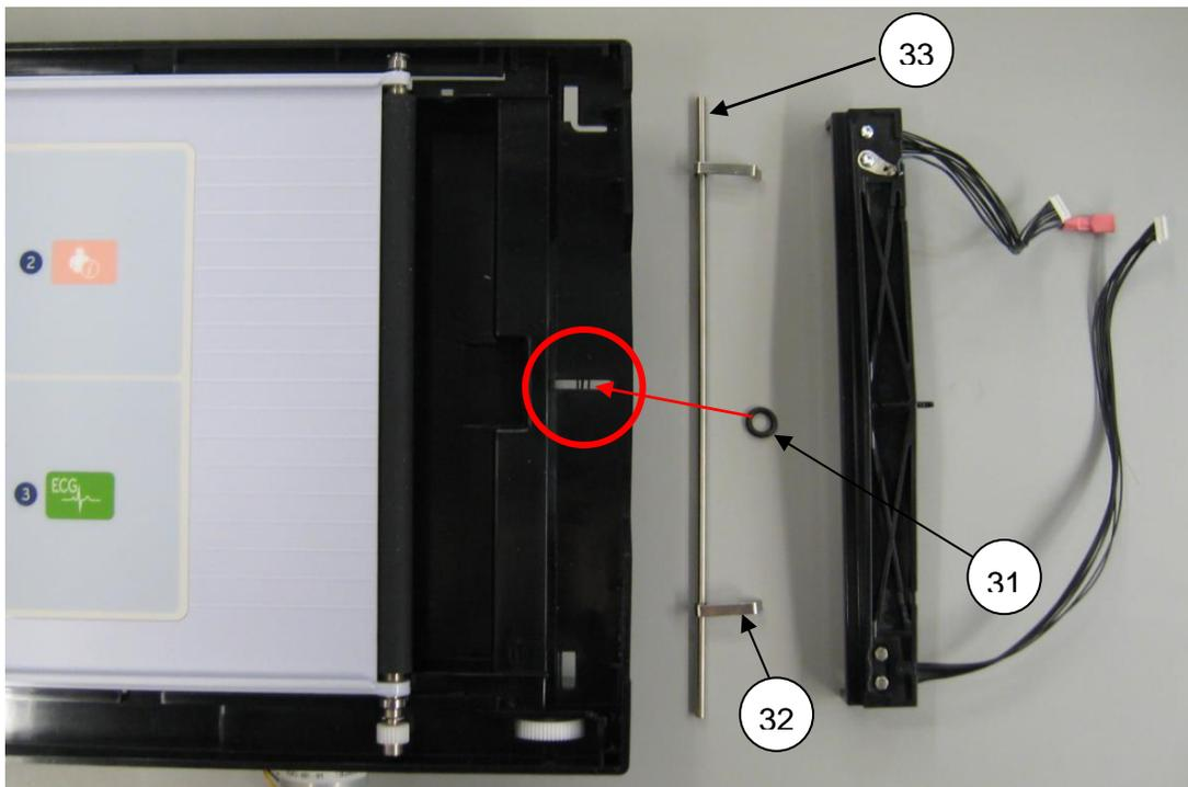
Once the printhead assembly is removed from its installed position, the Writer Door assembly can be removed by sliding it past the “closed” position until the removal/install slots are aligned. The door assembly is then lifted in an upward direction.
