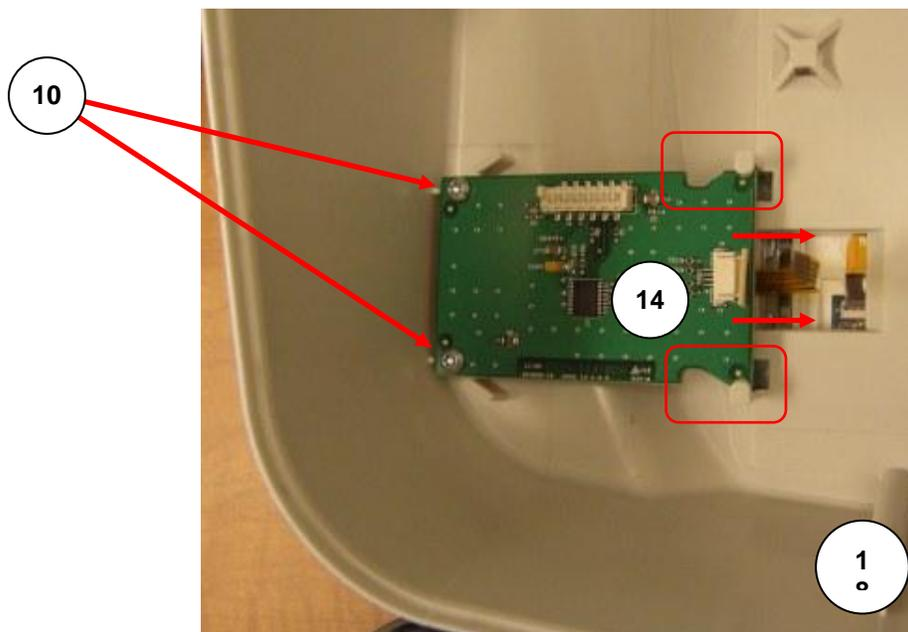
Remove the two T10 screws (item # 10) from the touch screen controller PCA, then slide the PCA over to allow the retaining hooks to pass through the slots in the PCA.
