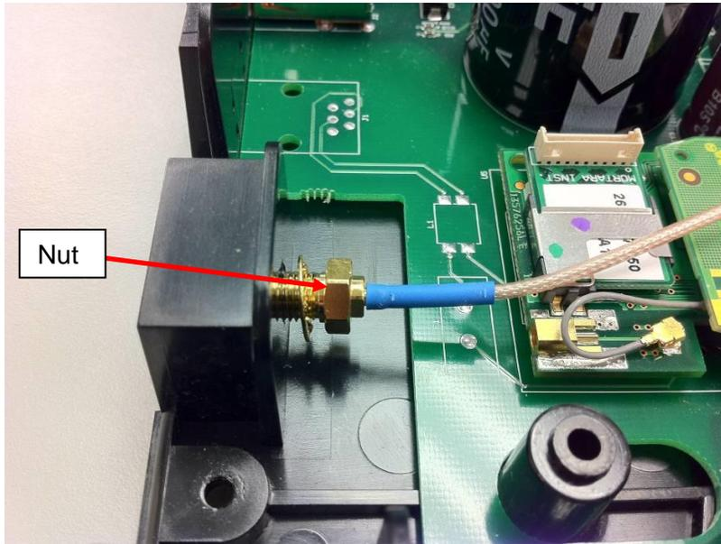
To install the assembly, first secure the antenna mount to the lower housing with the washer and nut using a 9.0 inch-pound hand torque wrench, and then connect the antenna cable to the communication module.
