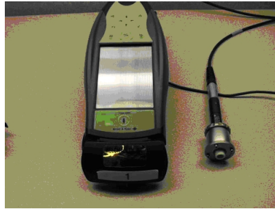
B&K sound level meter model 2250
