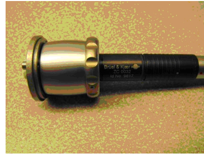
1/2-inch microphone model 4192 and 2 cc coupler model 4946
