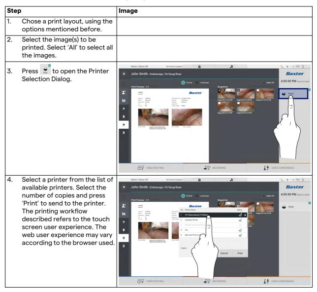
This function is available only after the selected printer(s) has/have been installed and configured on Helion by qualified service personnel.
