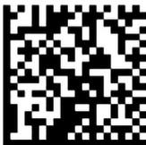
(01)00615521031626<br>(21)123456789012<br>(11)210212 | Indicates the Unique Device Identification (UDI) code; it is composed of:<br>– a device identifier (UDI-DI) (01);<br>– a production identifier (UDI-PI) (serial number (21), date of production (11)).                                                                                                                                                       |
