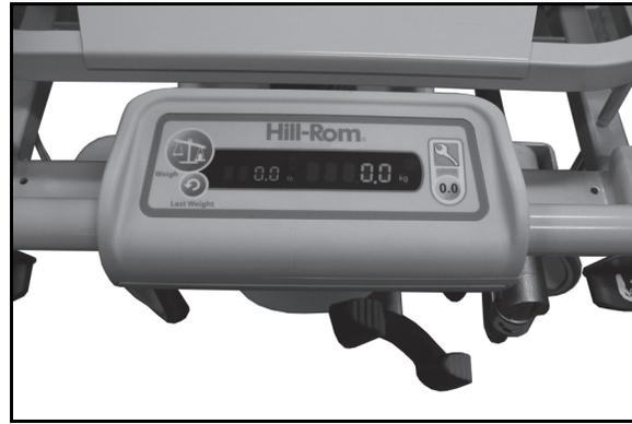
The scale system has an accuracy of 1% or 2.2 lb (1 kg), whichever is greater, and an operating range of 0 lb to 700.0 lb (0 kg to 317.5 kg). The scale control is at the foot end of the stretcher.
