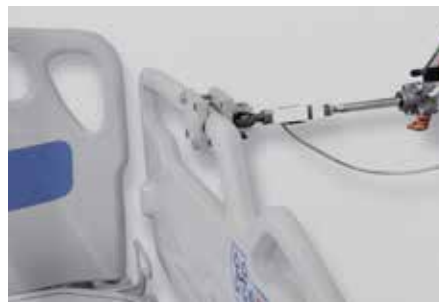
Push/Pull test on siderails
