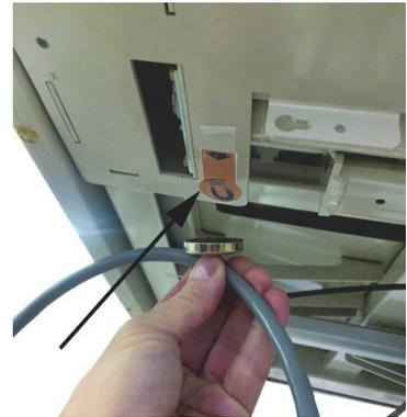
3. Attach the third magnet underneath the intermediate frame on the patient left-hand side of the bed.
