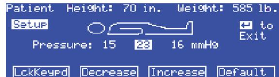
3. The unit automatically adjusts the pressures for the set height and weight. If necessary, use the arrow keys to move the cursor to the applicable pressure setting: head, seat, or foot, and adjust the settings as follows:
