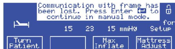
If the system meets the three bulleted conditions above and the powered width extensions still do not operate, the air supply unit may have an internal communication board error. If so, the **Communication Error** message will show.
