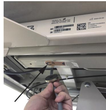
4. Attach the fourth magnet along the intermediate frame near the HiLo drive.
