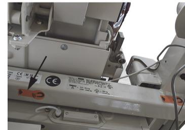
7. Attach the seventh magnet along the intermediate frame near the head-end of the bed.
