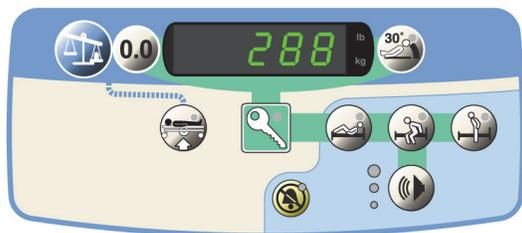
The scale system continuously weighs the patient; however, the weight does not continuously show on the display. You must press the Weigh control to view the patient's weight.
