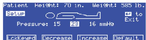
4. The unit automatically adjusts the pressures for the set height and weight. If necessary, use the arrow keys to move the cursor to the applicable pressure setting: head, seat, or foot, and use the Increase and Decrease controls to adjust the settings. To **return** all pressure settings to the pressures automatically set by the unit for the set height and weight, press **Default**.
