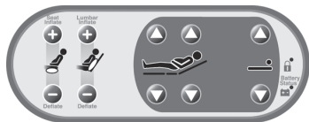
Panel de control del personal hospitalario
