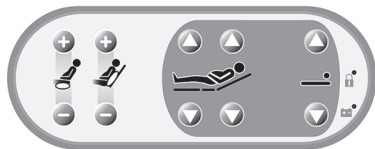
Panel de control del personal hospitalario
